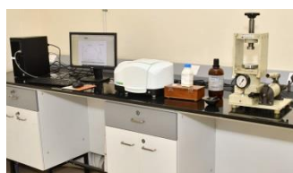
FTIR Spectrometer (Spectrum Two, Perkin Elmer)
