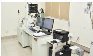
Mass High Resolution Field Emission Scanning Electron Microscope with EDS (FE-SEM)
