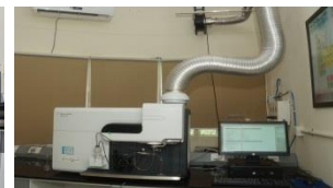
Microwave Plasma Atomic Emission Spectrometer (MP-AES Agilent 4210)
