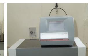
Microwave Synthesizer (Monowave 200, Anton Paar)
